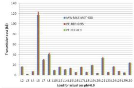
Fige 9. Transmission cost of each load with actual power factor of 0.9.
