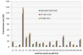
Fig. 8. Transmission cost of each load with actual power factor of 0.8
