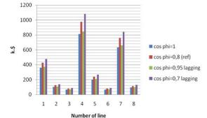
Fig. 4. The relationship between total costs  $(C_k,F_k,L_k)$  of the power factor in each line that contribute to the load # 2
