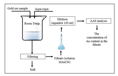
Figure 2. Design of leaching process
