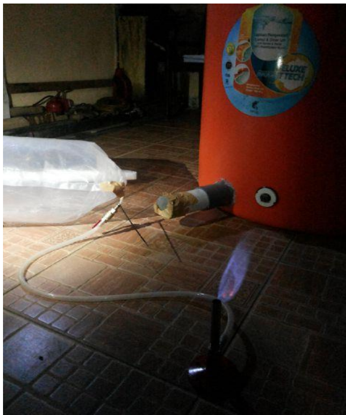
FIGURE 4. Biogas combustion test
