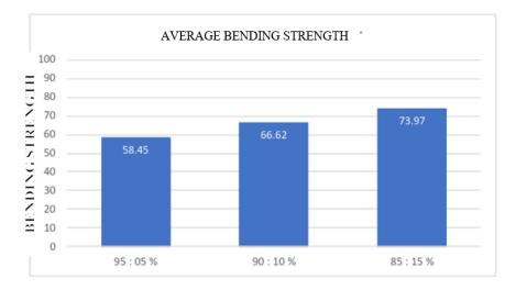
Figure 4. Average Bending strength for each weight fraction
