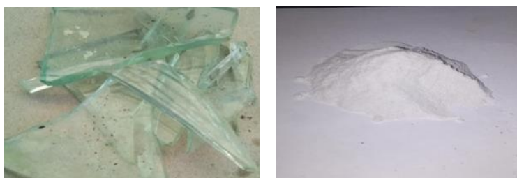
Figure 2. Photos of (a) glass waste and (b) glass waste powder.
