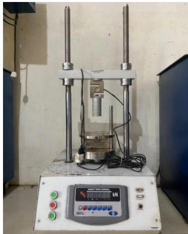
Gambar 3.1 : Indirect Tensile Strength
