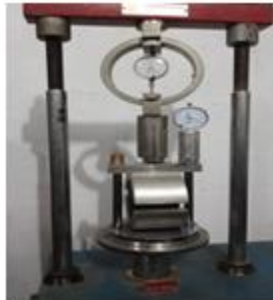
Figure 3. Marshall Test Equipment with test specimens (briquettes) for mixture testing
