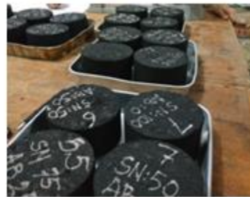
Figure 3. Marshall Test Equipment with test specimens (briquettes) for mixture testing
